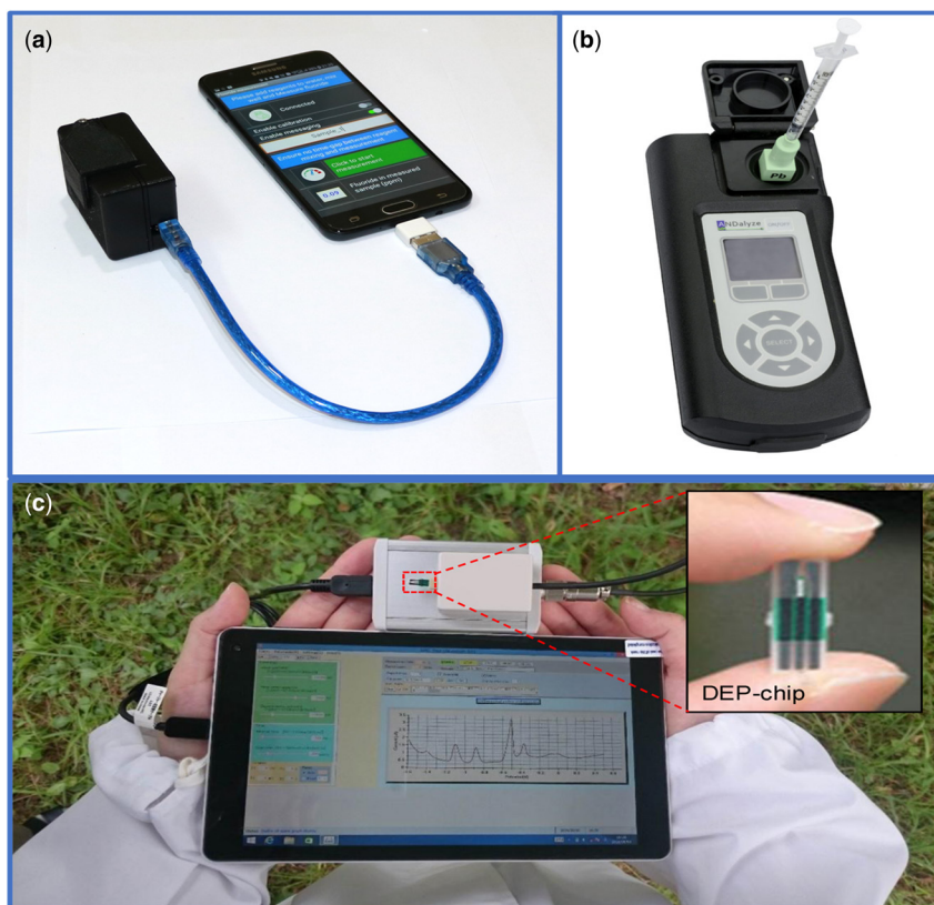
Figure 20.1 Portable devices developed for water quality analysis in field environments. (a) Smartphone based colorimeter for the testing of fluoride in groundwater (Mukherjee et al. , 2020). (b) AND 1100 Fluorometer utilised to determine toxicity levels of lead, copper, uranium, mercury, zinc, and cadmium (Reproduced with permission from Alpha Measurement Solutions). (c) DEP-On-Go (Biyani et al. , 2017).
