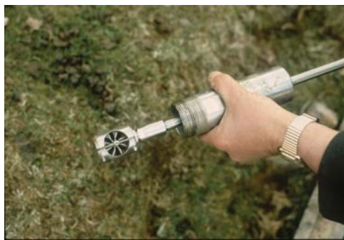
Figure 19 Typical insertion probes (Source: D Pearson (1, 2)).
