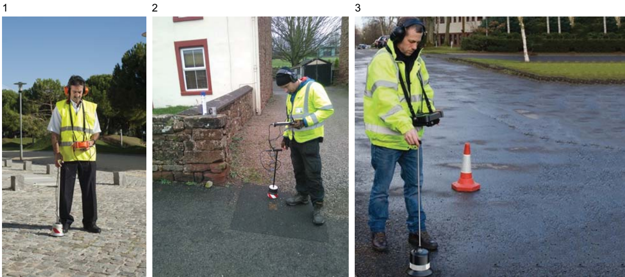
Figure 32 Photographs showing use of ground microphone (Sources: EPAL (Lisbon) (1), K Atkinson (2), S Hamilton (3)).
