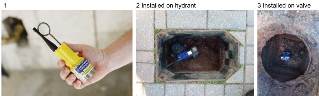
Figure 34 Photographs showing of acoustic loggers (Sources: EPAL (Lisbon) (1), K Atkinson (2, 3)).
