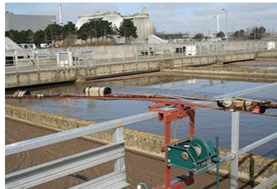
Figure 6.32: Field setup for measuring oxygen concentration profiles.
