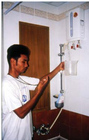
Figure 6.5 Conducting a residential audit and checking shower flow rate. Source: Maddaus Water Management (1995).
