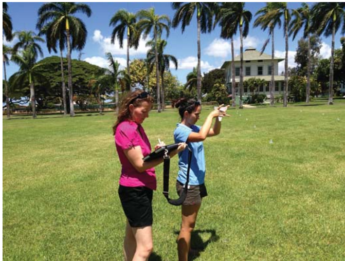
Figure 6.7 Recording data from a landscape water survey (catch can test) and entering data into a tablet computer to save time and increase accuracy. Source: Maddaus Water Management (2013).
