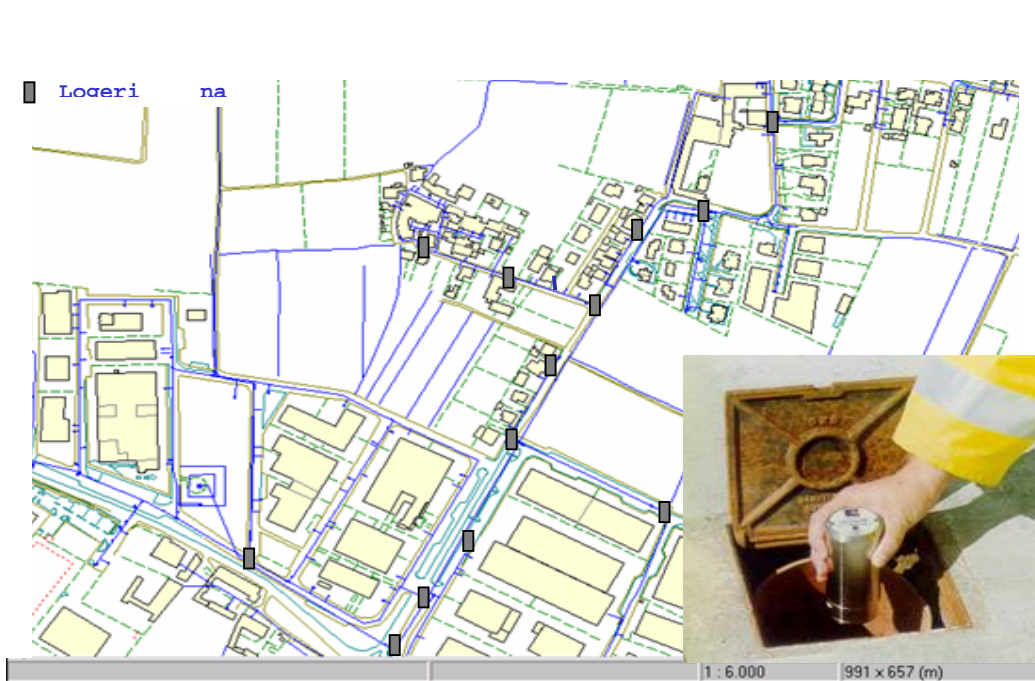
Figure 14: Acoustic logger placement in the distribution system
