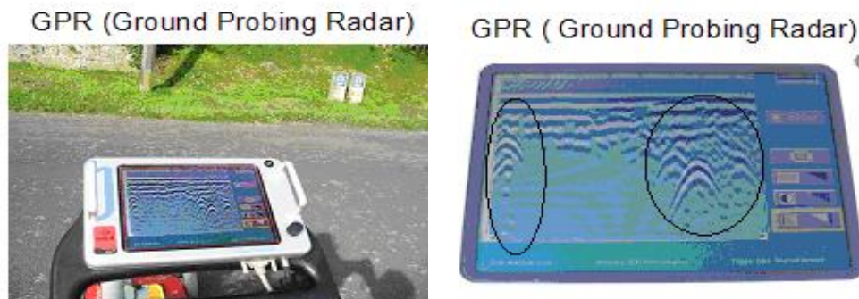
Figure 26: Leak Location using Ground Penetrating Radar
