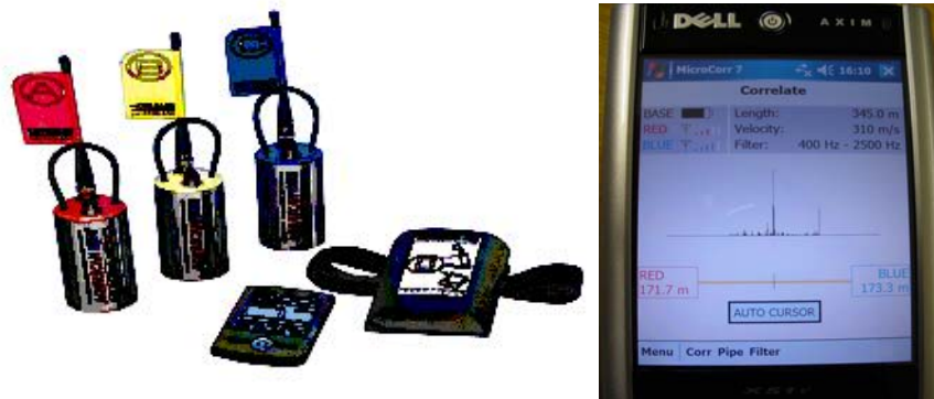
Figure 31: PDA based Correlator
