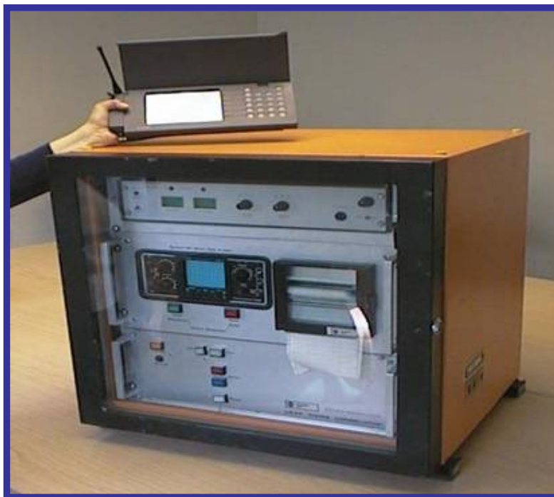
Figure 20: Leak Noise Correlator of the 1970s
