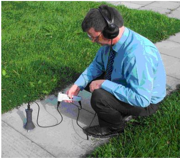
Figure 18: Leakage Engineer using a Ground Microphone
