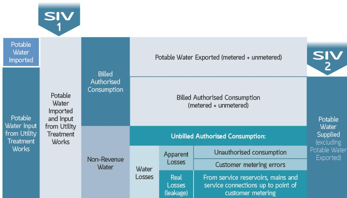
**Figure 8 – Simplified form of Standard IWA Annual Water Balance in Mm<sup>3</sup>.**
