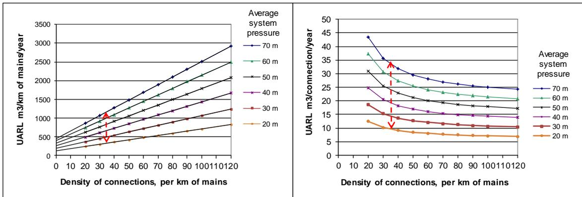
**Figure 7 – UARL in m<sup>3</sup>/km/year and m<sup>3</sup>/conn/year, for systems with customer meters 4m from mains.**
