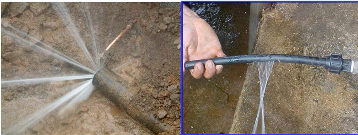
**Fixed Area leaks** – ring cracks, corrosion holes, blow-outs in rigid pipe materials.
