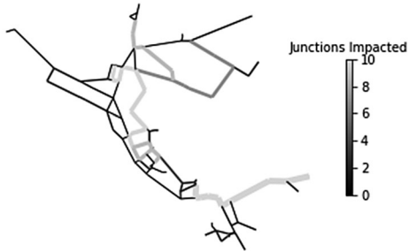
Figure 12.7 Net3 results from segment break analysis.
