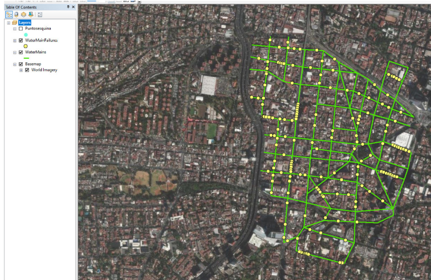
Figure 14.34 Water main grid with water main failures.
