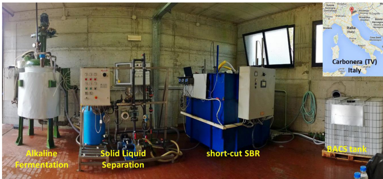
Figure 16.2 Pilot-scale S.C.E.N.A. system.
