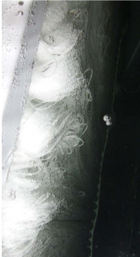
Figure 4.2 Photograph of gas permeable membranes covered with biofilm (provided courtesy of Oxymem.)
