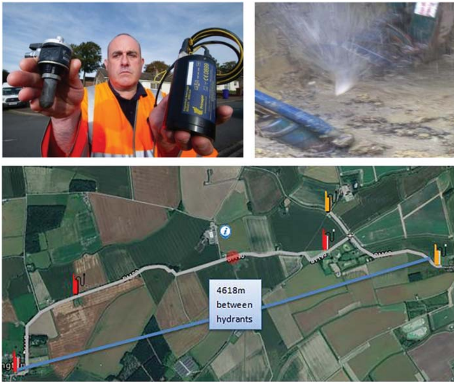
Figure 9.3 Remote correlating loggers with hydrophone sensors showing leak location (the red dot) over a distance of 4618 m. (Source: Anglian Water/Primayer)
