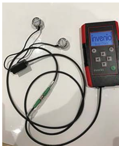
Figure 16.3 Vibration recorder. (Source: Invenio Systems)
