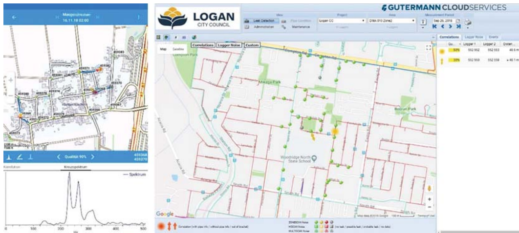
Figure 6.3 App for lift and shift correlation with upload function, cloud software to store and display individual measurements. (Source: Gutermann)
