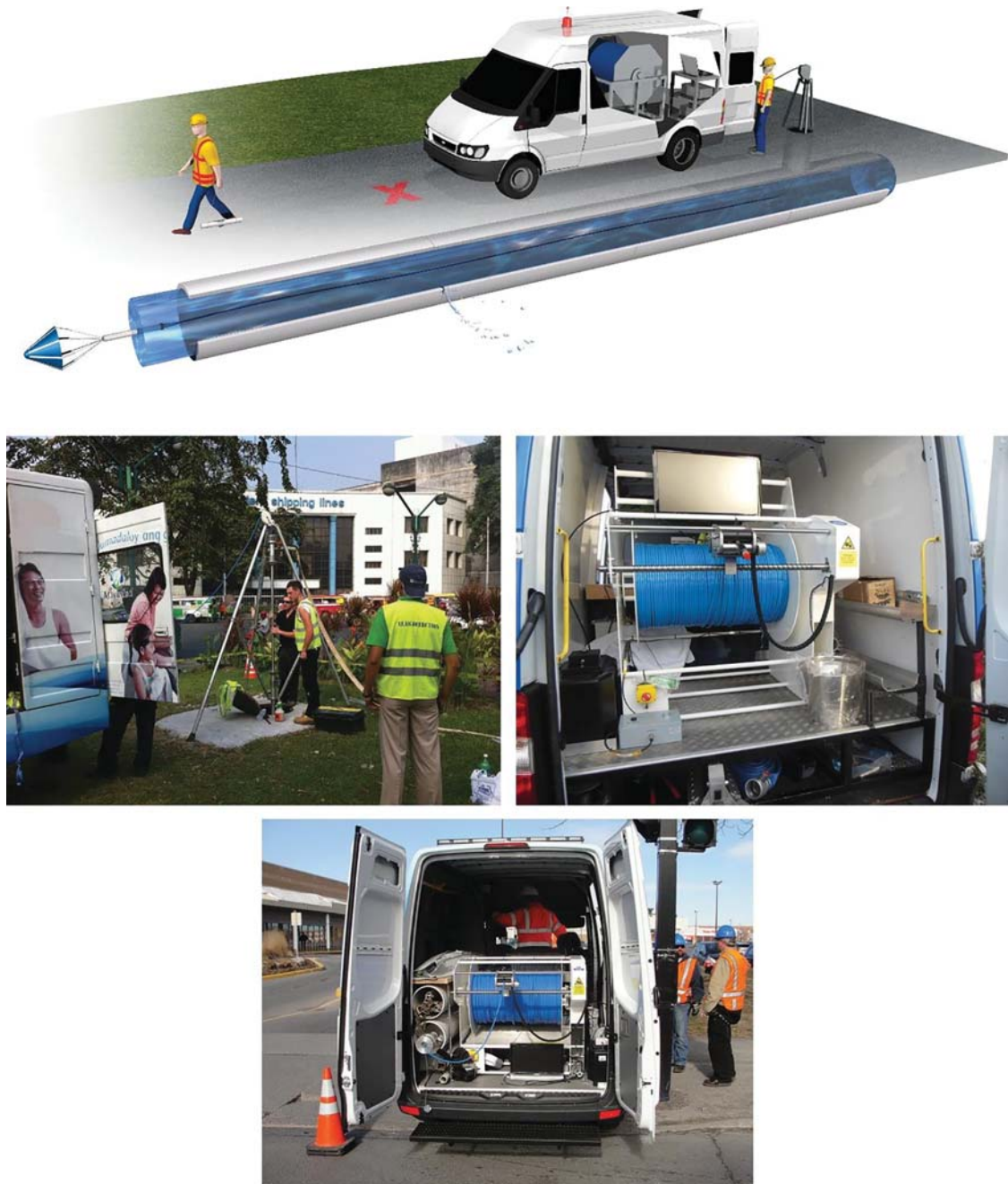
Figure 5.1 Tethered system access through 48 mm or above connection and only goes with the flow. (Source: Pure Technologies and JD7)
