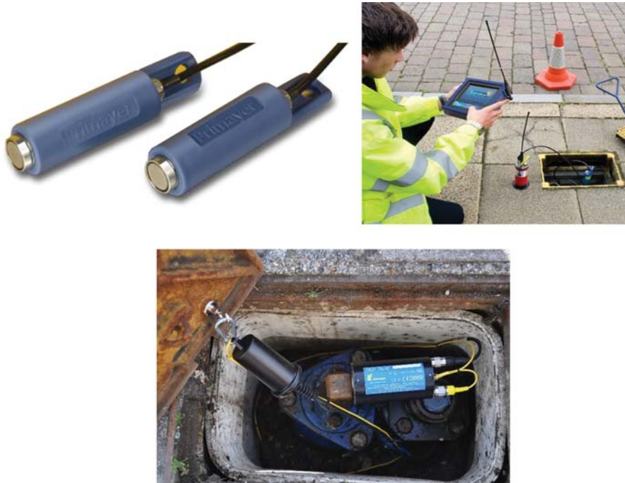
Figure 4.3 Examples of separate accelerometer sensors, as used with radio-base correlator and accelerometer integrated into correlating logger shown in lower picture. (Source: Primayer)
