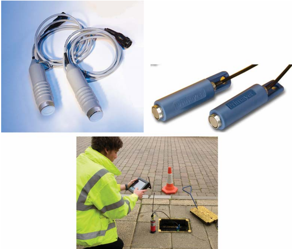
Figure 4.3 Example of Accelerometer (Source: Halma Water Management (left) and Primayer (right and bottom)).
