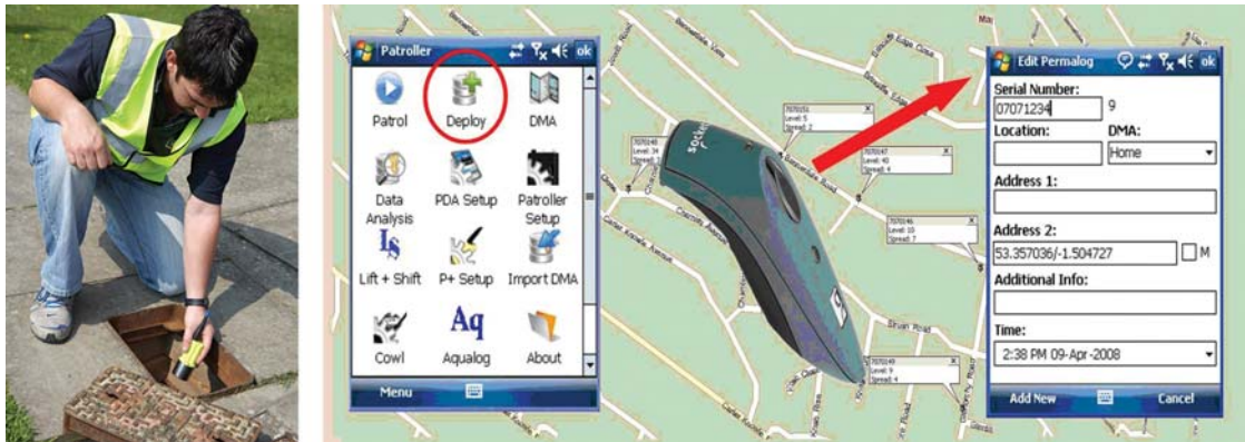
Figure 4.23 Lift and Shift Deployment and GPS Mapping Function (Source: Halma Water Management).
