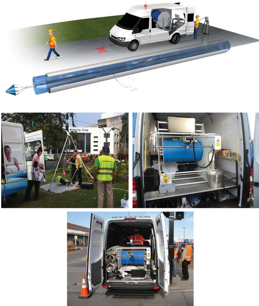
Figure 4.16 Tethered system access through 48 mm or above connection and only goes with the flow (Source: Pure Technologies and JD7).
