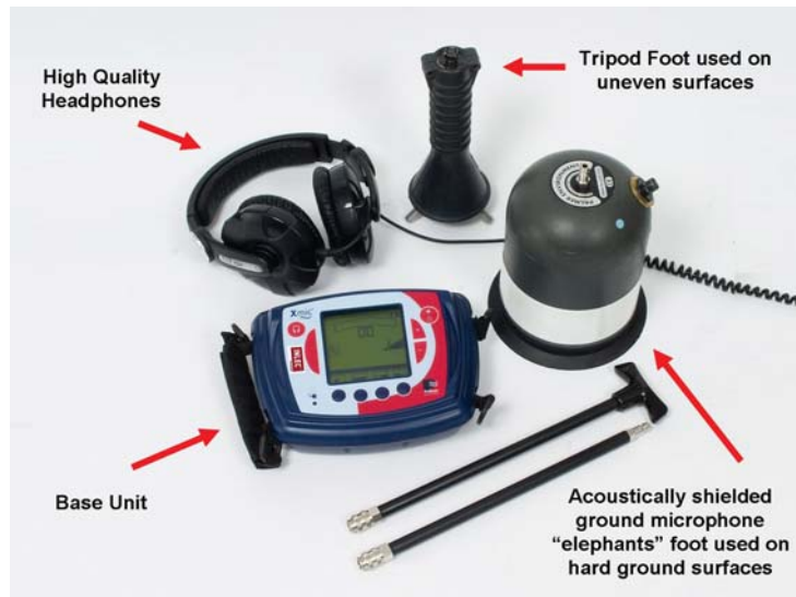
Figure 4.27 Components of Electronic Amplified Listening Device (Source: Halma Water Management).
