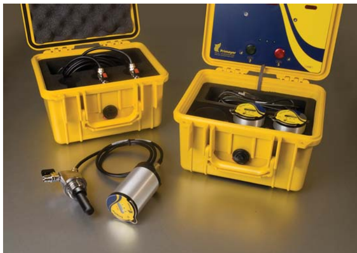
Figure 4.9 Correlating logger system with hydrophones (Source: Primayer).
