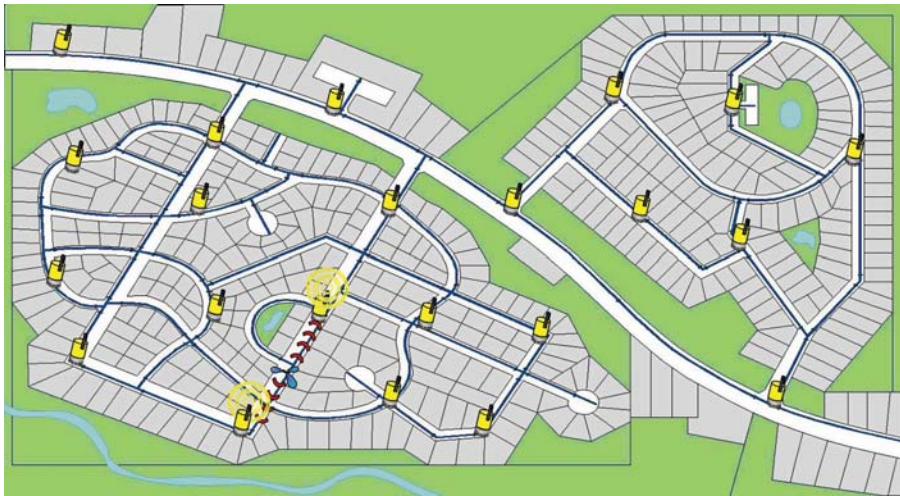
Figure 4.20 Noise logger schematic (Source: Halma Water Management).
