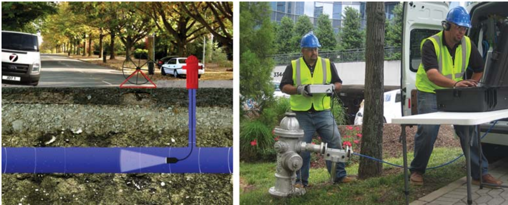
Figure 4.17 Push tethered system which can be operated with or against the water flow with access through tapping point or fire hydrant (Source: JD7).
