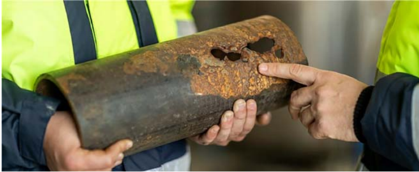
Figure CS8.2 Analysing leak holes in pipe samples.
